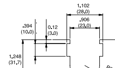
Recommended Panel Cut-Out
